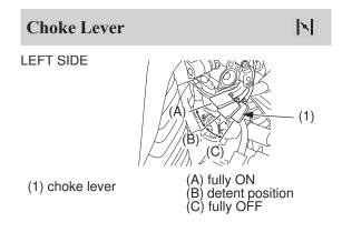
The choke lever (1) is used for starting the engine (page 31). The choke increases the percentage of fuel in the fuel/air mixture delivered to the engine.
