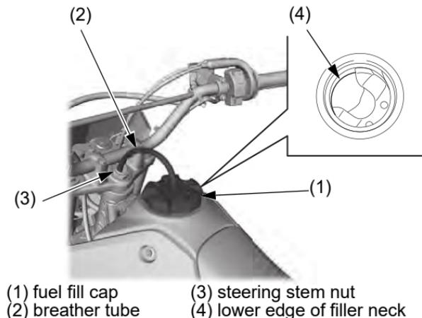
1. To open the fuel fill cap (1), pull the breather tube (2) out of the steering stem nut (3). Turn the fuel fill cap counterclockwise and remove it.
