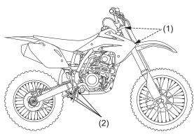
(1) steering head bearings(2) suspension pivot points
