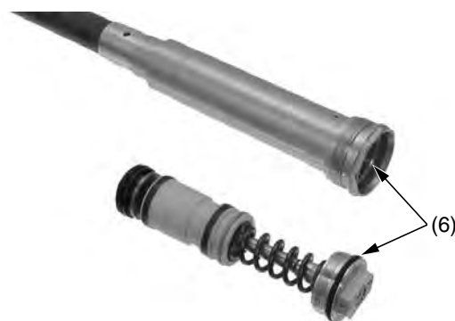
(6) fork cap and fork damper threads
