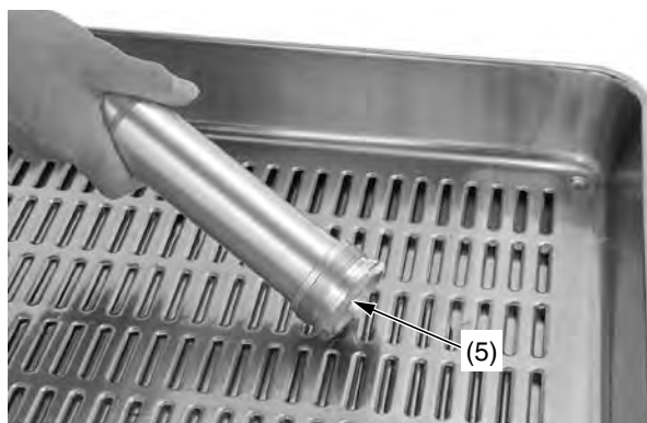
(5) fork damper oil/spring chamber
