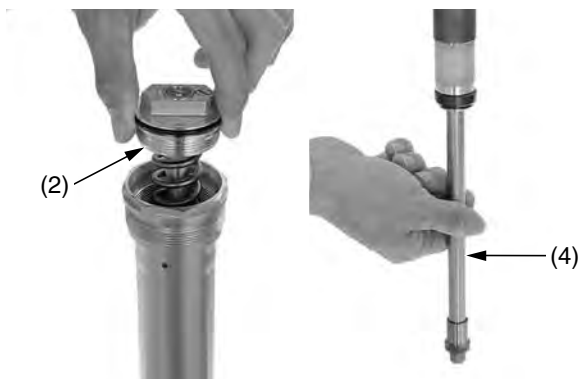
(2) fork cap assembly (4) fork damper piston rod
