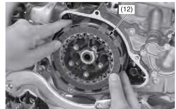
(12) clutch discs, clutch plates, judder spring and spring seat
