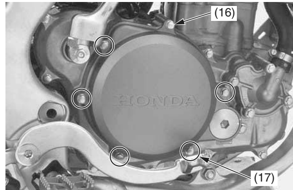
(16) clutch cover bolt A (17) clutch cover bolts B
