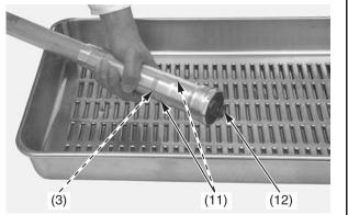
(3) fork damper oil chamber(11) oil holes(12) pressure release screw
