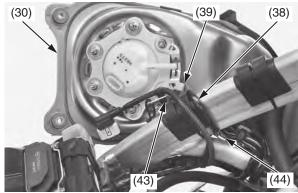
(30) fuel tank(38) stopper cable(39) stopper cable guide
