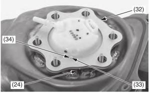
(24) dust seal lug(32) fuel pump plate(33) groove(34) fuel pump unit lug
