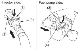
(2) fuel joint(3) slide retainer(4) connector housing
