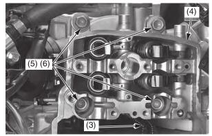
(3) cam chain(4) cylinder head(5) washers(6) cylinder head B bolts
