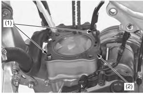
(1) dowel pins(2) cylinder head gasket (new)
