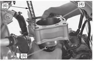
(4) cylinder bore(5) piston outer surface and piston rings(6) cam chain
