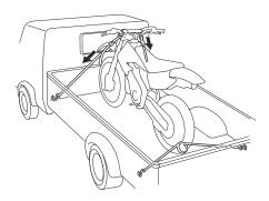
To secure your CRF, brace the front wheel against the front of the truck bed or trailer rail.
