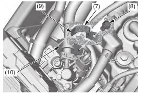
(7) clamp (8) bolt (9) clamp tab (10) groove 7. Install the fuel quick connect fitting cover (11).
