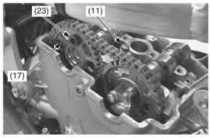
(11) rocker arm shaft stopper bolt(17) intake cam sprocket(23) cam sprocket bolt
