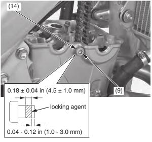
(9) sealing bolt(14) sealing washer (new)
