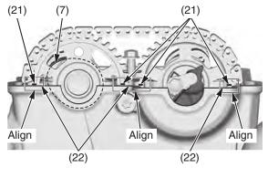
(7) camshaft cam lobe(21) timing marks(22) cylinder head mating surface
