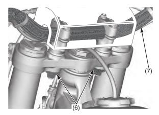
(6) handlebar lower holder nuts, washers and mounting rubbers
