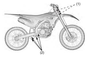
(1) steering head bearings(2) suspension pivot points
