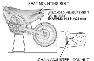
Measure the *loaded with rider* dimension. Remove the workstand. With two helpers available, sit as far forward as possible on your CRF's seat, wearing your riding apparel. Ask one helper to steady your CRF perfectly upright so you can put both feet on the pegs. Bounce your weight on the seat a couple of times to help the suspension overcome any situation and settle to a good reference point.
