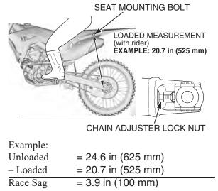
Calculate the *race sag* dimension. To do this, subtract the *loaded with rider* dimension (step 3) from the *unloaded* dimension (step 2). Standard Race Sag: 4.1 in (105 mm)
