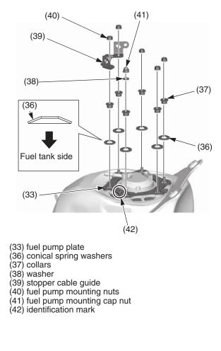
13. Tighten the fuel pump mounting nuts (40) and cap nut (41) to the specified torque in the specified sequence as shown:8 lbf·ft (11 N·m, 1.1 kgf·m)
