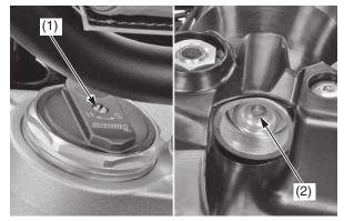
(1) compression damping adjuster(2) rebound damping adjuster
