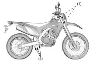
(1) steering head bearings(2) suspension pivot points
