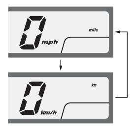
3. When selecting the "mph" and "mile" Press and hold SEL button. The speed and mileage unit is set, and then the display will return to the normal mode. <u>When selecting the "km/h" and "km"</u> Press and hold SEL button. The speed and mileage unit is set, and then the display moves the changing of the fuel mileage unit.
