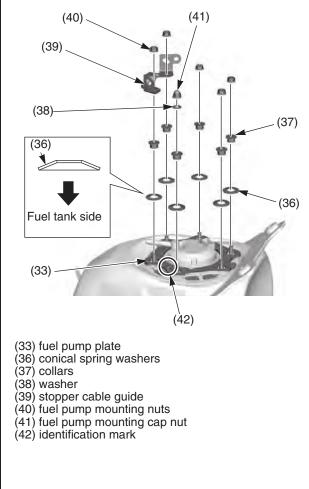
13. Tighten the fuel pump mounting nuts (40) and cap nut (41) to the specified torque in the specified sequence as shown:
