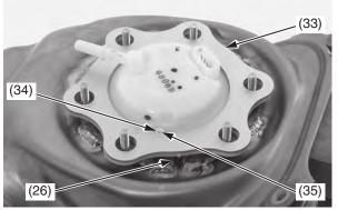
(26) dust seal lug(33) fuel pump plate(34) fuel pump plate groove(35) fuel pump unit lug
