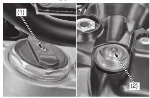
(1) compression damping adjuster(2) rebound damping adjuster
