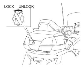
The travel trunk and saddlebags can be locked and unlocked with the ignition key or remote transmitter.
