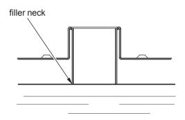
4. Add fuel until the level reaches the bottom of the filler neck. Avoid overfilling the tank. There should be no fuel in the filler neck.
