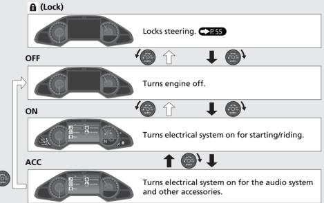
: Turning the ignition switch clockwise.
