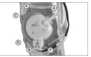
Install the fuel pump mounting bolts.
