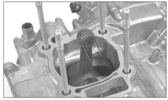
Measure the O.D. of the piston at 3.5 mm (0,1378 in) from bottom of skirt and 90 degrees to the piston pin hole.
