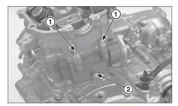
(1) CYLINDER HEAD BOLTS(2) CYLINDER SEALING BOLT
