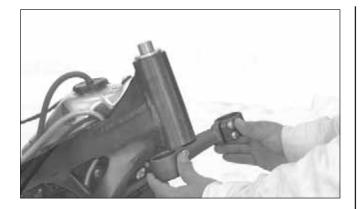
Turn the steering stem lock-to-lock 5 times to seat the bearings and retighten the adjusting nut to the specified torque.
