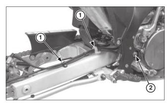
(1) BRAKE HOSE CLAMPS(2) SWINGARM PIVOT BOLT/NUT
