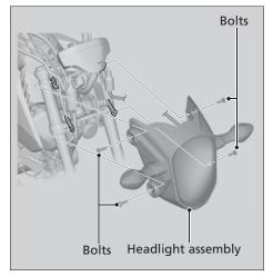
**1.** Remove the bolts and headlight assembly.
