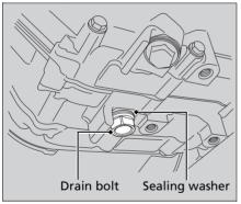
**6.** Install a new sealing washer onto the drain bolt. Tighten the drain bolt.
