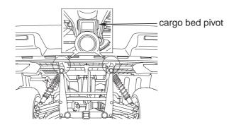
Lubricate the cargo bed latch pivots as shown in the following illustration.
