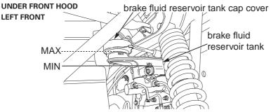
It should be between the MIN and MAX level marks. If the level is at or below the MIN level mark, check the brake pads for wear (page 142). 3. Return the brake fluid reservoir tank cap cover to its normal position.
