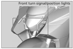
The front turn signal/position lights use several LEDs.
