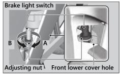
Check the operation of the brake light switch. Insert hands from front of the front lower cover hole.
