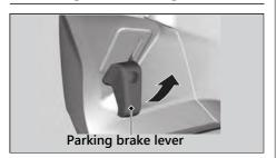
Place your motorcycle on a firm, level surface. Stop the engine and push your motorcycle while set the parking brake to check the efficacy of the parking brake.
