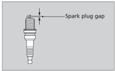
**8.** Install the spark plugs. With the plug washers attached, thread the spark plugs in by hand to prevent cross-threading.
