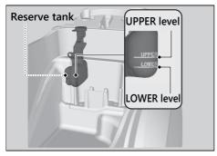
If the coolant level is dropping noticeably or the reserve tank is empty, you likely have a serious leak. Have your vehicle inspected by your dealer.
