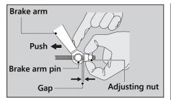
After adjustment, confirm the freeplay of the brake lever.
