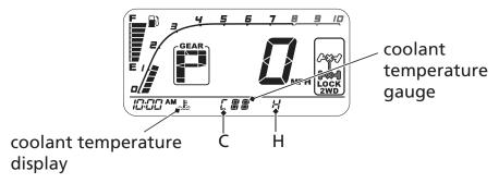
If all sections of the coolant temperature gauge, including segment H and high coolant temperature indicator are on (automatically appears in the display), stop the engine and check the reserve tank coolant level.
