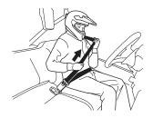
To unlatch a seat belt, press the red PUSH button on the buckle.
