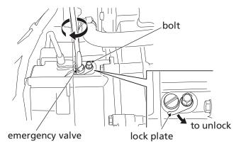
3. Return the lock plate and tighten the bolt securely.
