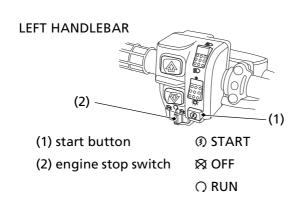
The start button (1) is used for starting the engine. Pushing the button in starts the engine. See *Starting Procedure*, page 52.
