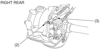
(2) brake lever adjusting nut (3) brake arm pin
