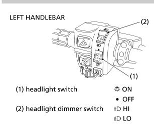
The headlight switch (1) is used to turn the headlight ON  $(\clubsuit)$  or OFF  $(\bullet)$ . To operate, turn the switch to ON  $(\clubsuit)$  or OFF  $(\bullet)$ .
