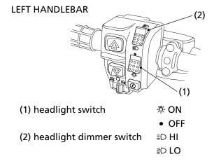
The headlight switch (1) is used to turn the headlight ON ( $\mathfrak{P}$ ) or OFF ( $\bullet$ ). To operate, turn the switch to ON ( $\mathfrak{P}$ ) or OFF ( $\bullet$ ).
