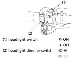
The headlight switch (1) is used to turn the headlight ON ( $\mathfrak{P}$ ) or OFF ( $\bullet$ ). To operate, turn the switch to ON ( $\mathfrak{P}$ ) or OFF ( $\bullet$ ).
