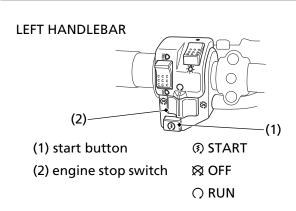
The start button (1) is used for starting the engine. Pushing the button in starts the engine. See *Starting Procedure*, page 50.
