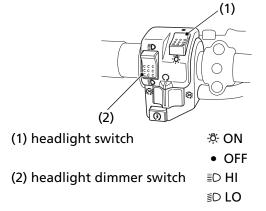
The headlight switch (1) is used to turn the headlight ON ( $\mathfrak{P}$ ) or OFF ( $\bullet$ ). To operate, turn the switch to ON ( $\mathfrak{P}$ ) or OFF ( $\bullet$ ).
