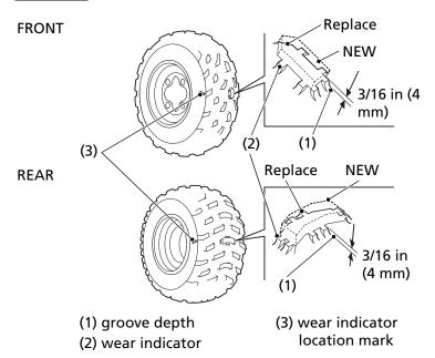
To check the condition of a tire tread, measure the groove depth (1) in the center of the tire, or check the wear indicator (2). For best performance, you should replace a tire before the tread depth at the center reaches the following limits:
